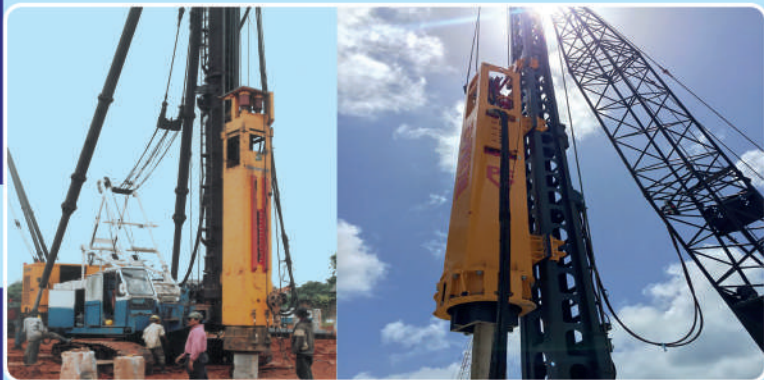
Impact Hammer; Brand: Twinwood, Model: V100D; Self Weight: 13.5 Ton; Hammer Capacity: 10 Ton
