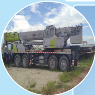
70 Ton Mobile Crane; Brand: Zoomlion; Model: ZLJ5481JQZ70V; Capacity: 70 Ton; Boom: 46 M; Fly Jib: 16 M; Year: 2016
