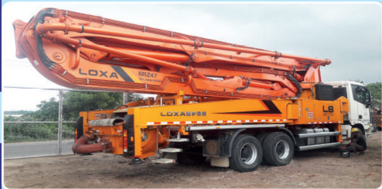
Concrete Pump Truck; Brand: LOXA; Model: 6RZ47; Capacity: 60m 3 /hr; Boom Length: 47 M
