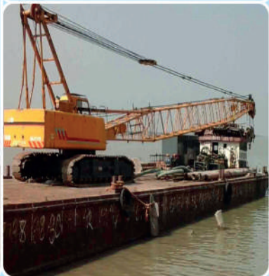
70 Ton Crawler Crane; Brand: Kobelco; Model: 7070 1F; Capacity: 70 Ton; Boom: 57 M; Fly Jib: 18 M
