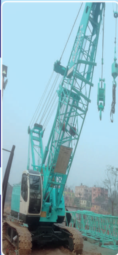
55 Ton Crawler Crane; Brand: Kobelco; Model: 7055-3F; Capacity: 55 Ton; Boom: 51 M; Fly Jib: 16 M
