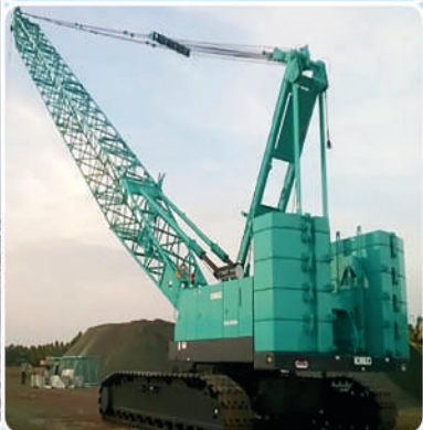
150 Ton Crawler Crane; Brand: KOBELCO; Model: 7150; Capacity: 150 Ton; Boom: 73.15 M; Fly Jib: 30.48 M
