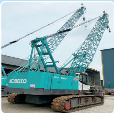
80 Ton Crawler Crane; Brand: KOBELCO; Model: CKE800; Capacity: 80 Ton; Boom: 54.86 M; Fly Jib: 18.29 M
