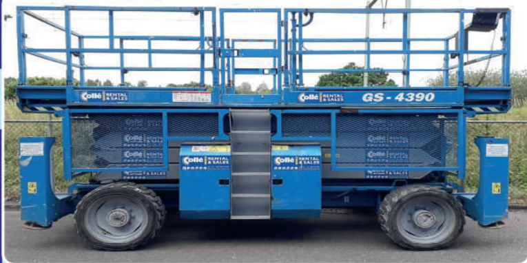
14.75 Meter Scissor Man Lift; Brand: GENIE; Model: GS4390; Lifting Capacity: 14.75 M; Load Capacity: 680 K.G.
