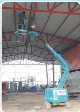
6 Meter Man Lift; Brand: NAGANO; Model: NUL06; Lifting Capacity: 6 M; Load Capacity: 100 K.G.
