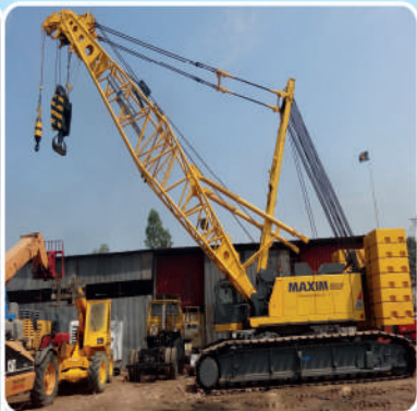
280 Ton Crawler Crane; Brand: Hitachi Sumitomo; Model: SCX2800-2; Capacity: 280 Ton; Boom: 72 M; Fly Jib: 30 M
