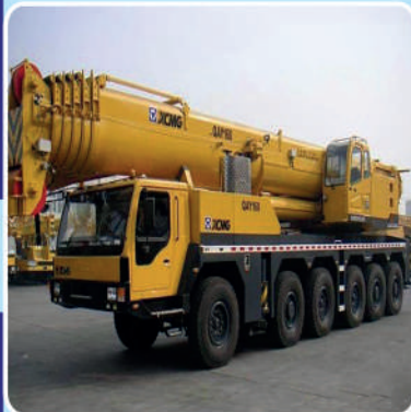
160 Ton Mobile Crane; Brand: XCMG; Model: QAY160; Capacity: 160 Ton; Boom: 56.3 M; Fly Jib: 24 M
