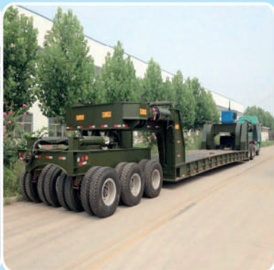
Multi Axle Hydraulic Modulator 150 Ton Low Bed Trailer; Brand: Titan; Model ALP4591
