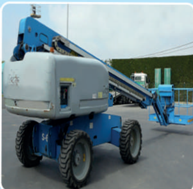
40 Meter Man Lift; Brand: Genie; Model: S125; Lifting Capacity: 40 M; Load Capacity: 230 K.G.
