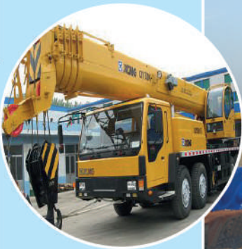
50 Ton Mobile Crane; Brand: XCMG; Model: QY50KA; Capacity: 50 Ton; Boom: 43.5 M; Fly Jib: 11.4 M; Year: 2015
