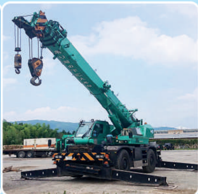
35 Ton Mobile Crane; Brand: TADANO; Model: GR350N-1; Capacity: 35 Ton; Boom: 36.3 M; Fly Jib: 8 M
