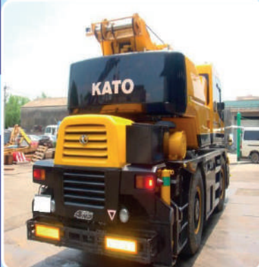
25 Ton Mobile Crane; Brand: KATO; Model: SR-250VR; Capacity: 25 Ton; Boom: 30.5 M; Fly Jib: 13 M
