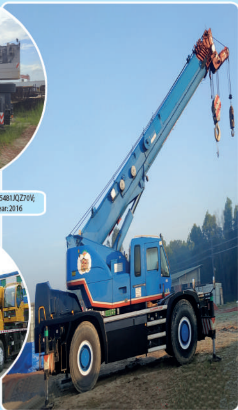
51 Ton Mobile Crane; Brand: KATO; Model: KR-50H-L2; Capacity: 51 Ton; Boom: 43 M; Year: 2006
