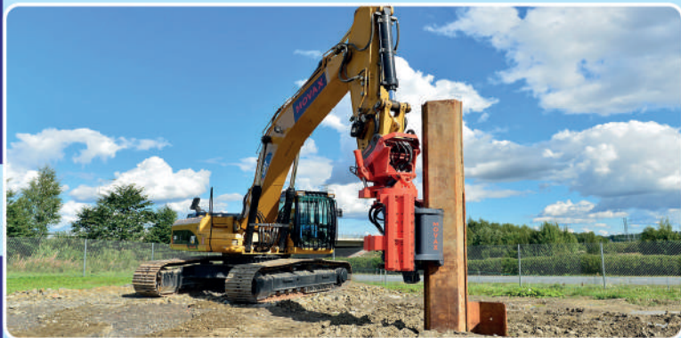
Pile Driver Excavator; Brand: CAT; Model: MKTV-5ESC; Pile Length: 18M; Boom Load: 10 Ton
