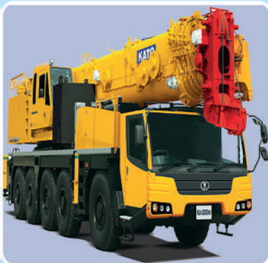
100 Ton Mobile Crane; Brand: KATO; Model: KA-1000; Capacity: 100 Ton; Boom: 45 M
