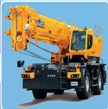
45 Ton Mobile Crane; Brand: KATO; Model: KR 45 HV; Capacity: 45 Ton; Boom: 39 M; Fly Jib: 14.5 M
