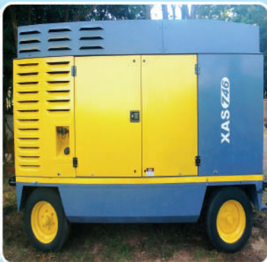
Air Compressor; Brand: Atlas Copco; Capacity: 750 CFM
