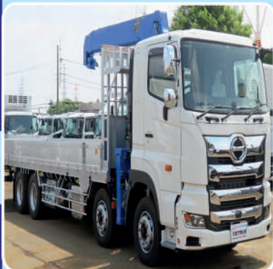
Truck Mounted Crane; Brand: Hino; Model: SK373, Capacity: 5 Ton
