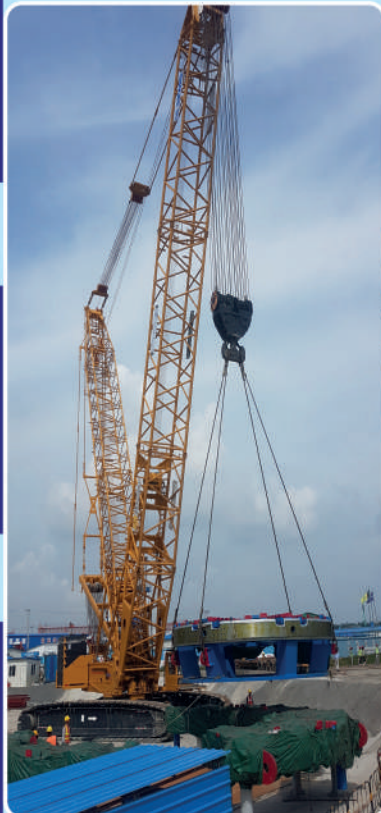
500 Ton Crawler Crane; Brand: XCMG; Model: QUY 500; Capacity: 500 Ton; Boom: 84 M; Fly Jib: 24 M
