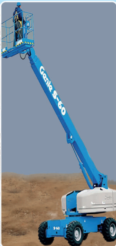
18 Meter Man Lift; Brand: GENIE; Model: S-60/34; Lifting Capacity: 18 M; Load Capacity: 227 K.G.
