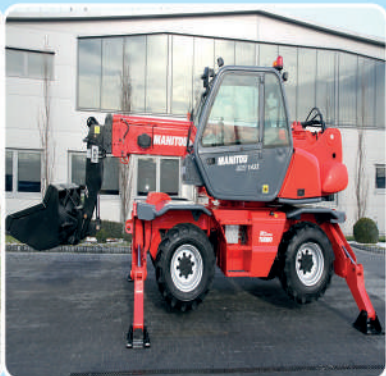
3.2 Ton Telescopic Fork Lift; Brand: Manitou, France; Model: MRT 1432; Load: 3.2 Ton; Lifting Height: 14 M
