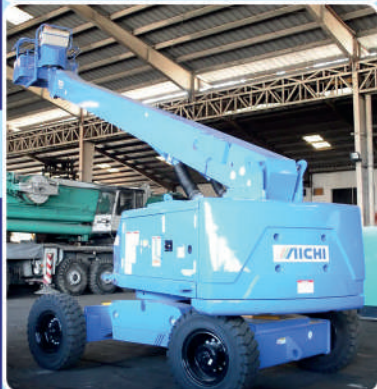
22 Meter Man Lift; Brand: AICHI; Model: SK 22 A; Lifting Capacity: 22 M; Load Capacity: 200 K.G.
