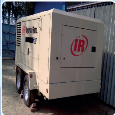
Air Compressor; Brand: Ingersoll Rand; Capacity: 750 CFM
