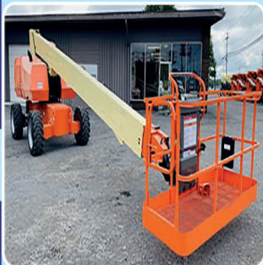
32 Meter Man Lift; Brand: JUNJIN; Model: T 320 N; Lifting Capacity: 32 M; Load Capacity: 250 K.G.
