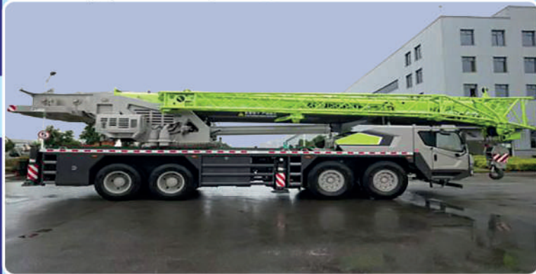
80 Ton Mobile Crane; Brand: ZoomLion; Model: ZLJ5502JQZ80V; Capacity: 80 Ton; Boom: 50 M; Fly Jib: 17.5 M
