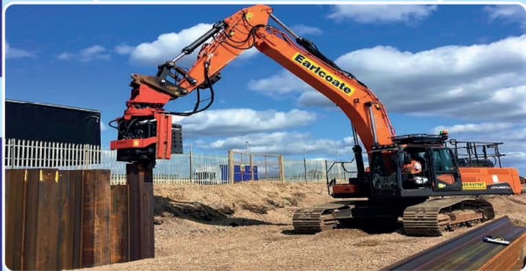
Pile Driver Excavator; Brand: Doosan; Model: DX-380; Pile Capacity: 13M; Boom Load: 7 Ton
