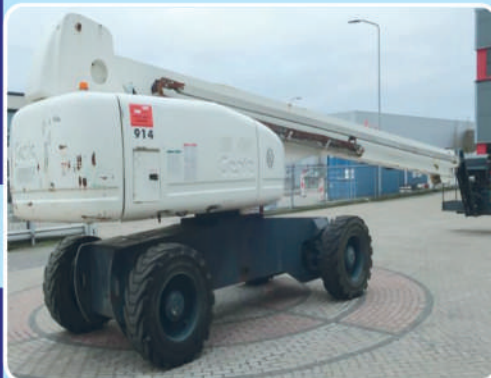
34 Meter Man Lift; Brand: GENIE; Model: S105; Lifting Capacity: 34 M; Load Capacity: 270 K.G.
