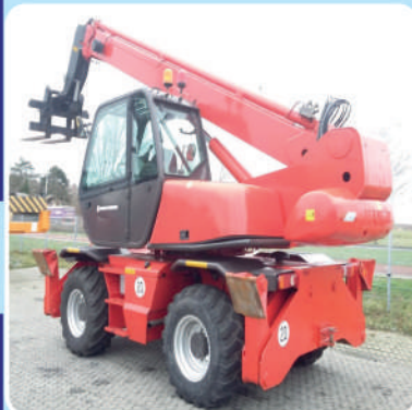
3.3 Ton Telescopic Fork Lift; Brand: Manitou, France; Model: MRT 1033; Load: 3.3 Ton; Lifting Height: 10 M
