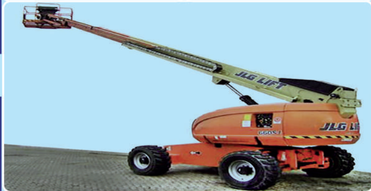
26 Meter Man Lift; Brand: JLG; Model: 660 SJ; Lifting Capacity: 26 M; Load Capacity: 249 K.G.
