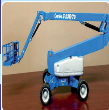
43 Meter Man Lift; Brand: Genie; Model: Z-135/70; Lifting Capacity: 43M; Load Capacity: 300 K.G.
