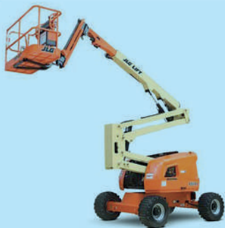
30 Meter Man Lift; Brand: JLG; Model: 800 AJ; Lifting Capacity: 30 M; Load Capacity: 236.80 K.G.
