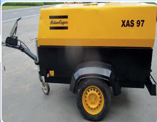
Air Compressor; Brand: Atlas Copco; Capacity: 100 CFM
