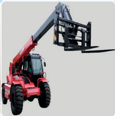
3.5 Ton Telescopic Fork Lift; Brand: MANITOU; Model: MRT-1635; Load: 3.5 Ton; Lifting Height: 16 M
