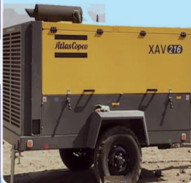
Air Compressor; Brand: Atlas Copco; Capacity: 450CFM
